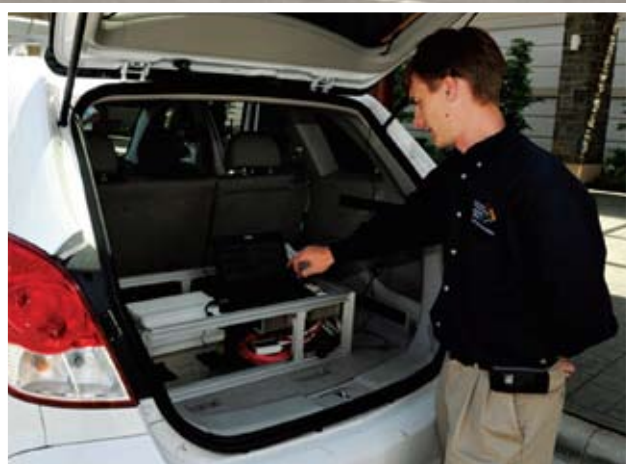
Three vehicles equipped with GPS, a DSRC radio, a computer and a monitor were used to demonstrate SwRI's advanced vehicle safety platooning application at the ITSA annual meeting in Washington, D.C.
