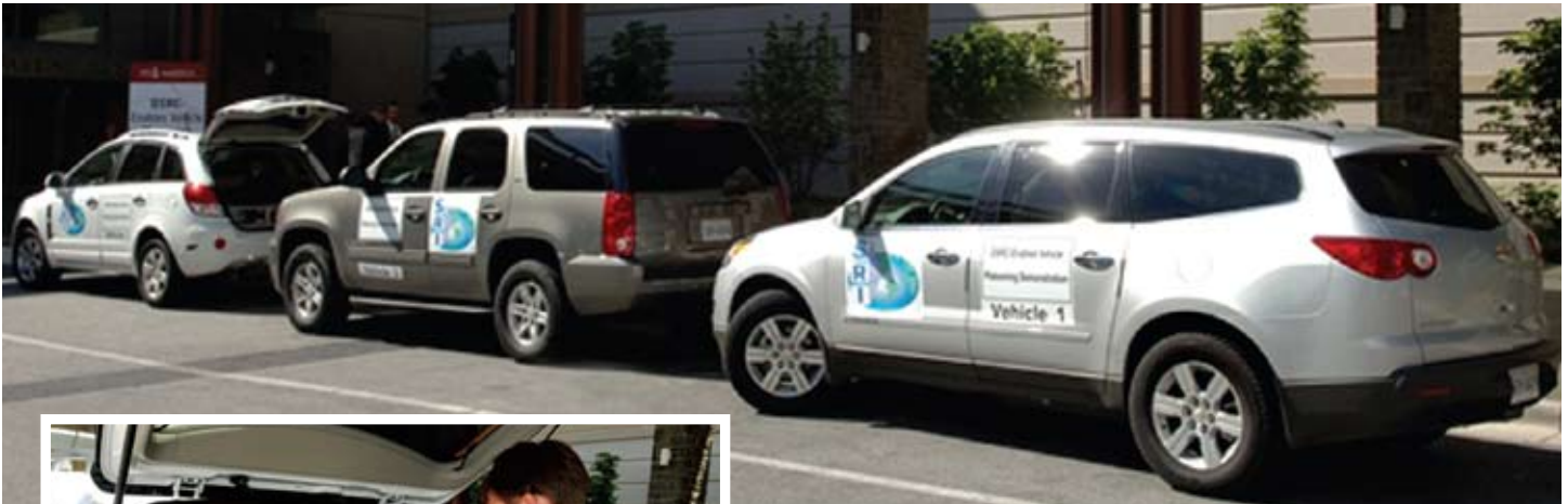
Three vehicles equipped with GPS, a DSRC radio, a computer and a monitor were used to demonstrate SwRI's advanced vehicle safety platooning application at the ITSA annual meeting in Washington, D.C.
