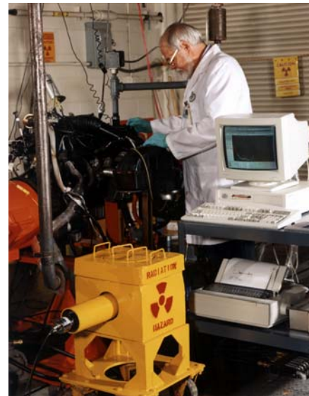
Figure 2. Engine and Detector in Engine Test Cell
